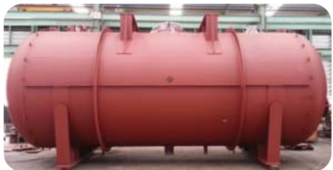
Oxygen Removal Tank
