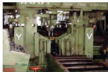
Automatic Drilling Machine Capacity :- Max. Dimension of Work piece are 1 M. for Side Drill, and 350 mm. for Top Drill
