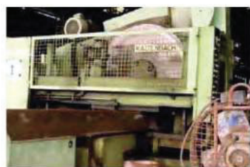
Circular Sawing Machine Capacity :- Max. Dimension of Work piece are 0.4 M.(H) x 1 M.(W)
