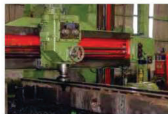
Shape & Milling Machine Capacity :- Max. Dimension of Work piece 1 M.(H) x 1.5 M.(W) x 4 M.(L)
