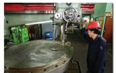
Radial Drilling Machine Capacity :- Arm = 1.8 M. Dia. = 50 mm.
