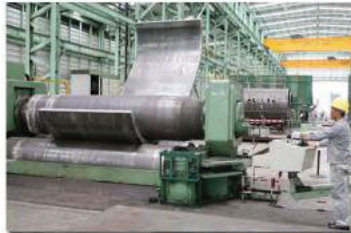
Plate Bending Machine Capacity :- Max. 3.1 M. Span Min. Dia. 600 mm. Max. Thickness = 50 mm.
