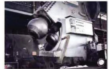
Cold Forming Flange Machine Capacity :- Max. Dia = 3.8 M. Max. Thickness = 22 mm.
