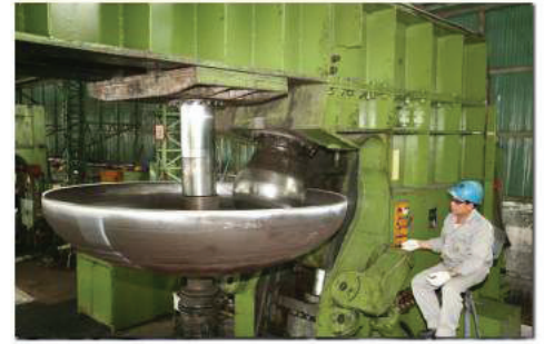
Cold Forming Flange Machine Capacity :- Max. Dia. = 6 M. Max. Thickness = 40 mm.
