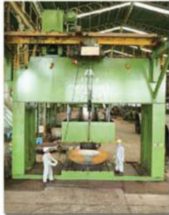
Hydraulic Press Capacity :- Max. Load = 1500 tons Max. 6M Spand
