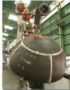
Welding Manipulator Capacity :- Max. 4.3 M. Arm 4.5 M. Height
