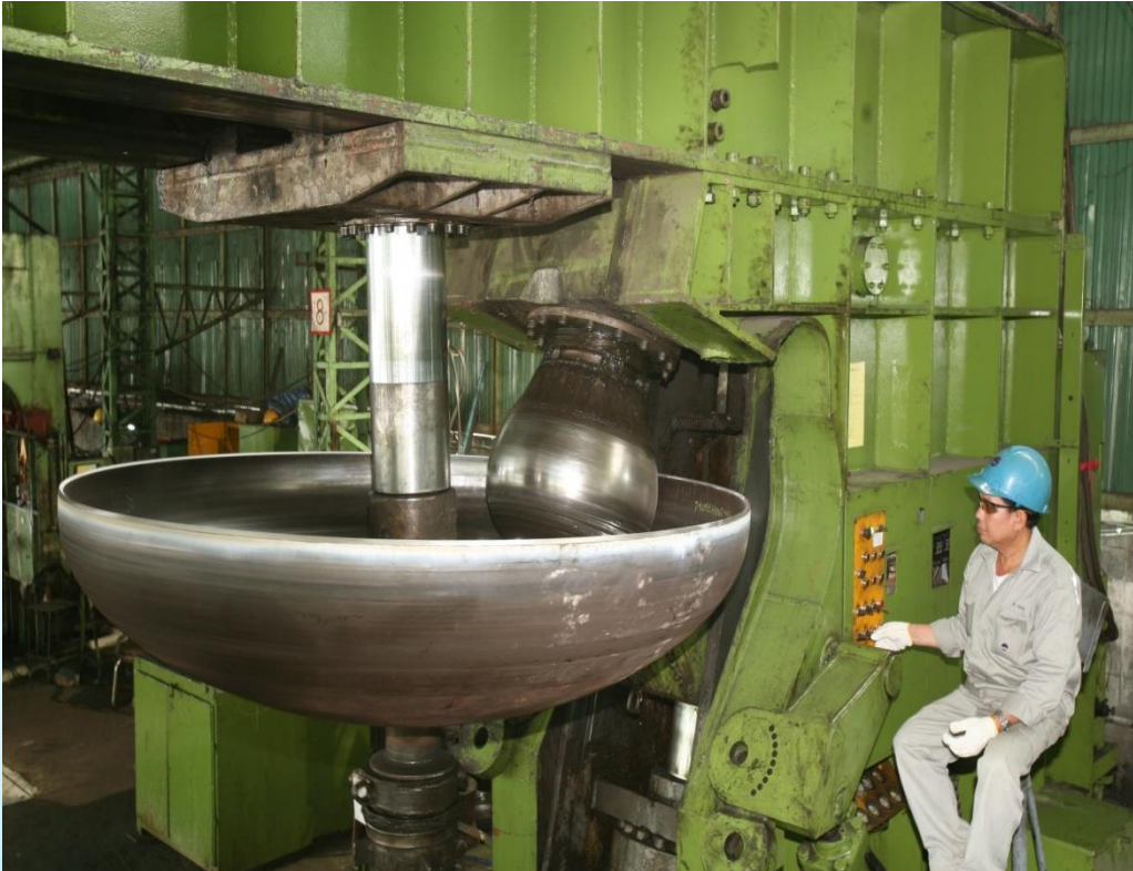
Cold forming machine: Max diameter: 6 m. Max thickness: 40 mm.
