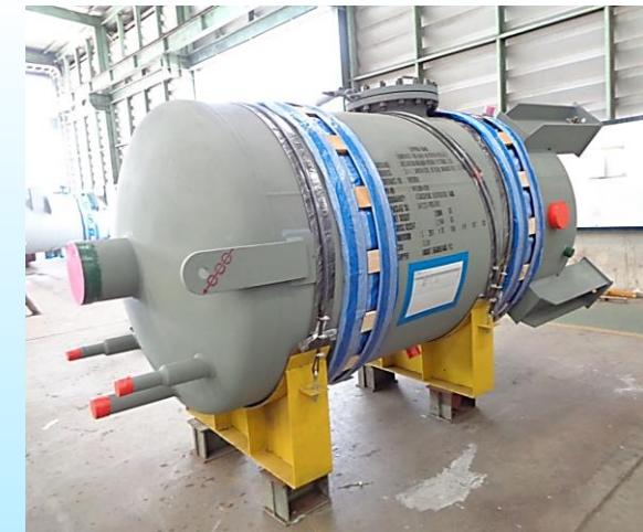
Blow Down Tank
