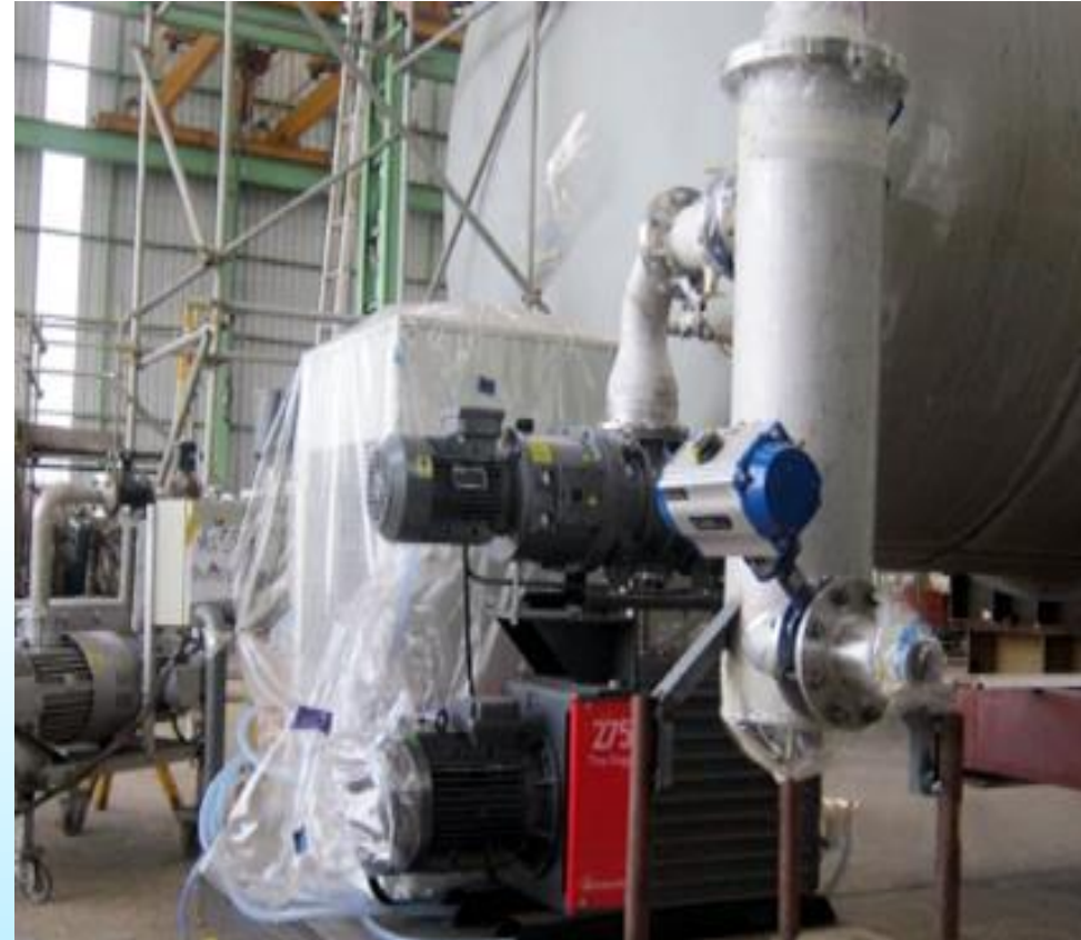
Vacuum pump w/ Booster E2M275 EH1200 Rotary pump speed: 275 m 3 /hr. Booster pump speed: 1200m 3 /hr.
