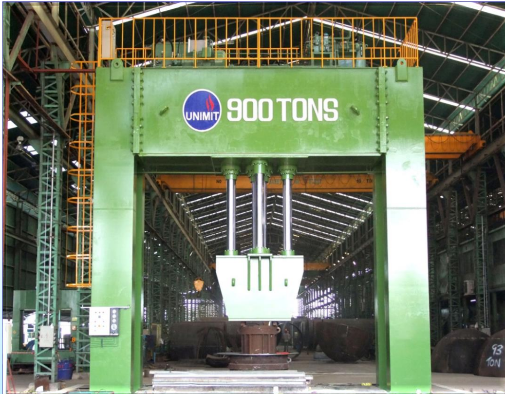
Pressing Capacity Max. Force 900 Tons Column Span 6000 mm. (inside)
