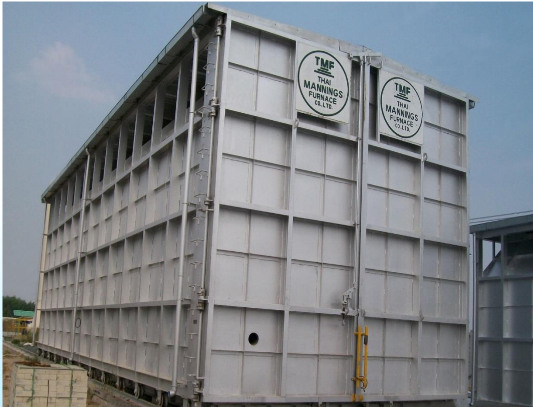
Capacity: 5.3 m.(W) x 5.3 m.(H) x 18.0 m.(L) 100 Tons Up to 1,200 C degree (LPG-fired)
