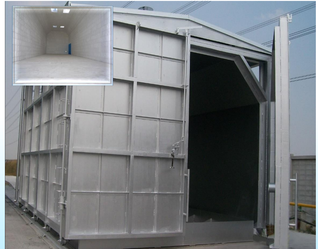
Capacity: 4.5 m.(W) x 3.5 m.(H) x 6.5 m.(L) 50 – 60 Tons Up to 1,200 C degree (LPG-fired)
