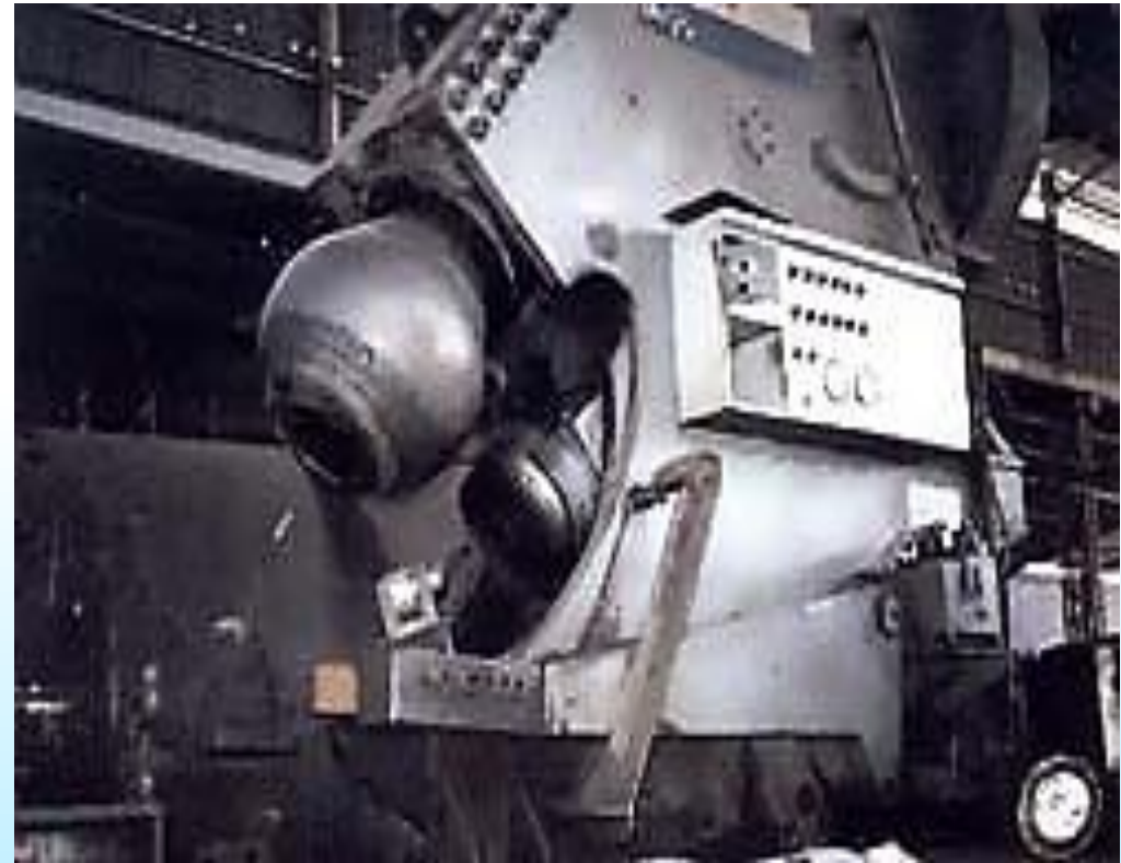
Cold forming machine: Max diameter: 3.8 m. Max thickness: 22 mm.
