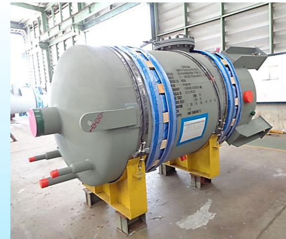
Blow Down Tank
