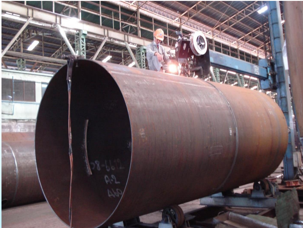
Semi-Automatic Longitudinal Welding with Manipulator
