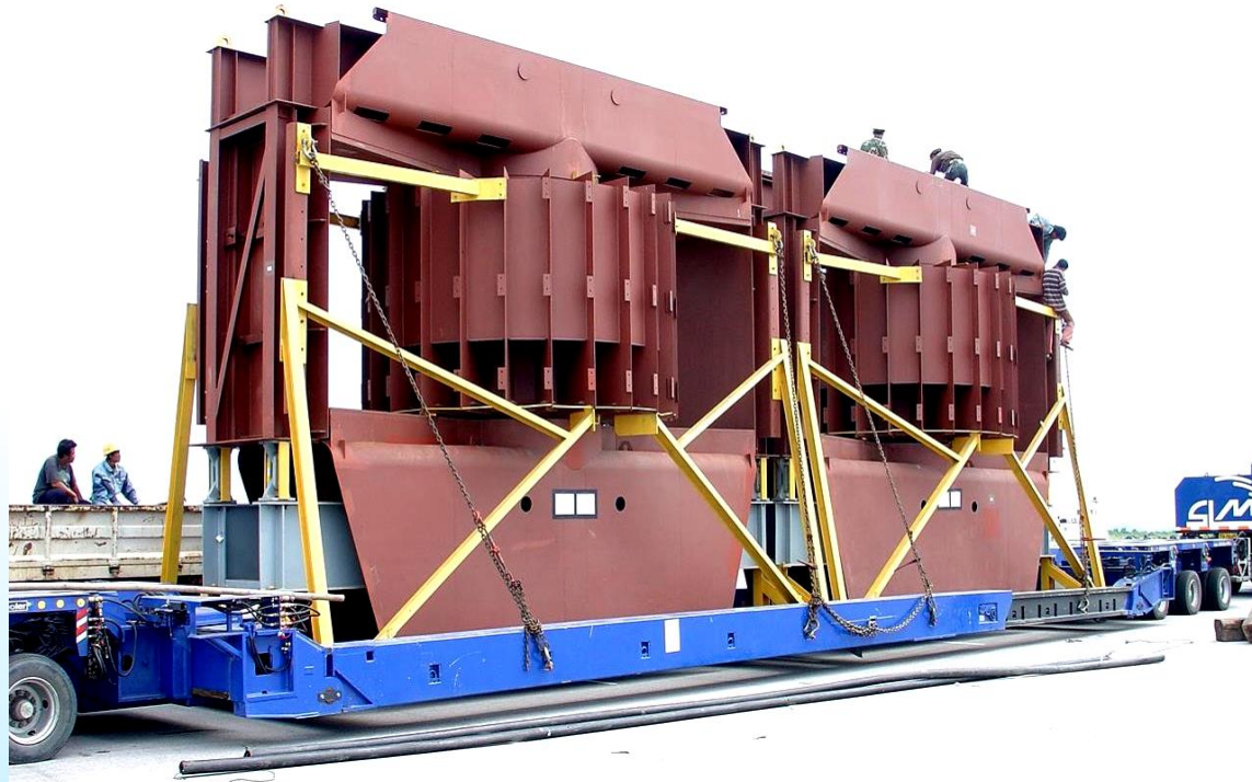
Boiler Fan Casing, Rotors & Static Parts
